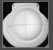
Measurement of lens position, diameter and orientation
