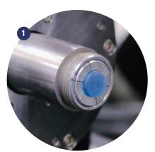
A 12.7 mm (0.500") diameter collet is recommended for all Boston® products (1). The pressure of the collet on the periphery of the button material is a critical factor that should be controlled. Excessive collet pressure can cause base curve warpage and/or stability problems. The collet closure mechanism should be adjusted for minimum pressure on the button, while still sufficiently holding the button during the lathing process.
