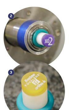
An alternate method of lathing the base curve is to block the button onto a flattopped arbor (2). This approach ensures there is no excessive collet pressure exerted on the button material.
